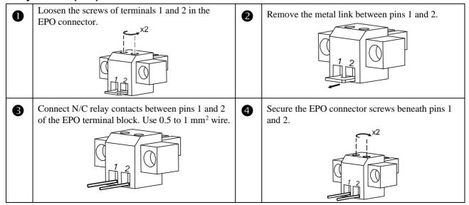
**NOTE:** If the N/C is open, the UPS will turn off and power will be removed from the load.
